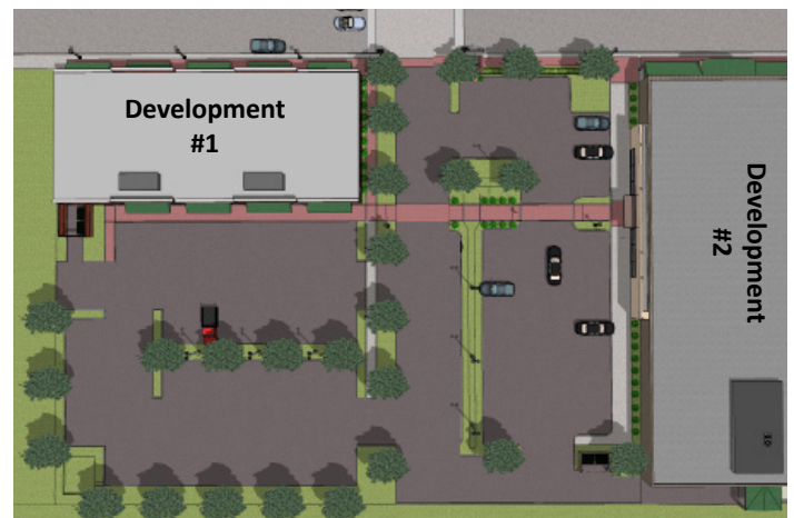
The above concept illustrates shared parking between two developments connected by an access drive, and includes vegetative buffers along all pedestrian routes.
