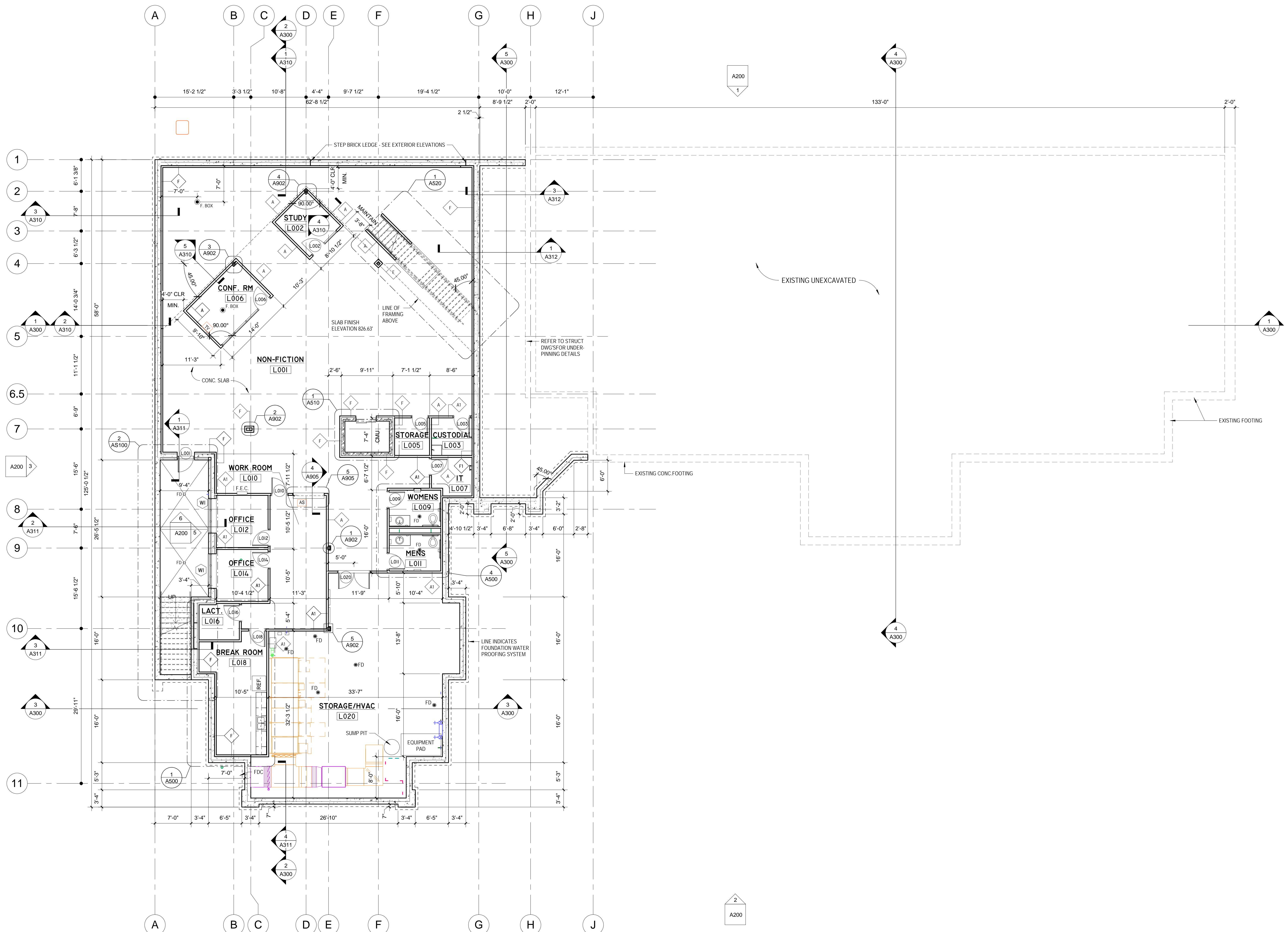
1 LOWER LEVEL CONSTRUCTION PLAN 1/8" = 1'-0"
